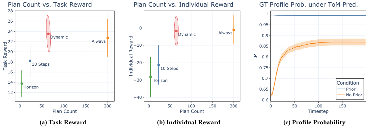
Figure 4: (a)–(b): impact of various replanning schemes on the agents’ task and individual cumulative rewards. Covariance ellipses represent the 95% CI of the mean. (c): mean probability over the course of trials of the ground-truth profile of the teammate under the ToMnet prediction in the presence ( Prior ) vs. absence ( No Prior ) of prior information about the teammate.
